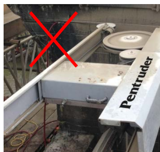
In this setup there is a lot of friction on the slack side.
