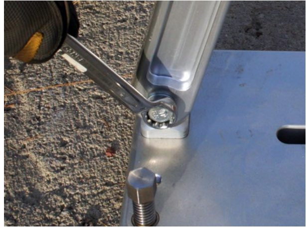
b. Loosen the lower bolt on the back support.
